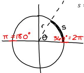
When s = r, we say that the corresponding angle  $\theta$  which is subtended by arc s has measure 1 radian.
